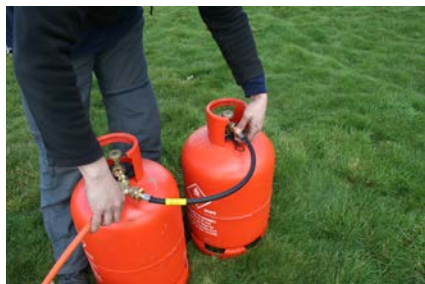
7. Offer up the gas assembly to the bottles. Hand tighten the threaded connector to the gas. Position bottles upwind of the beacon. NOTE: Propane is a reverse thread to tighten
